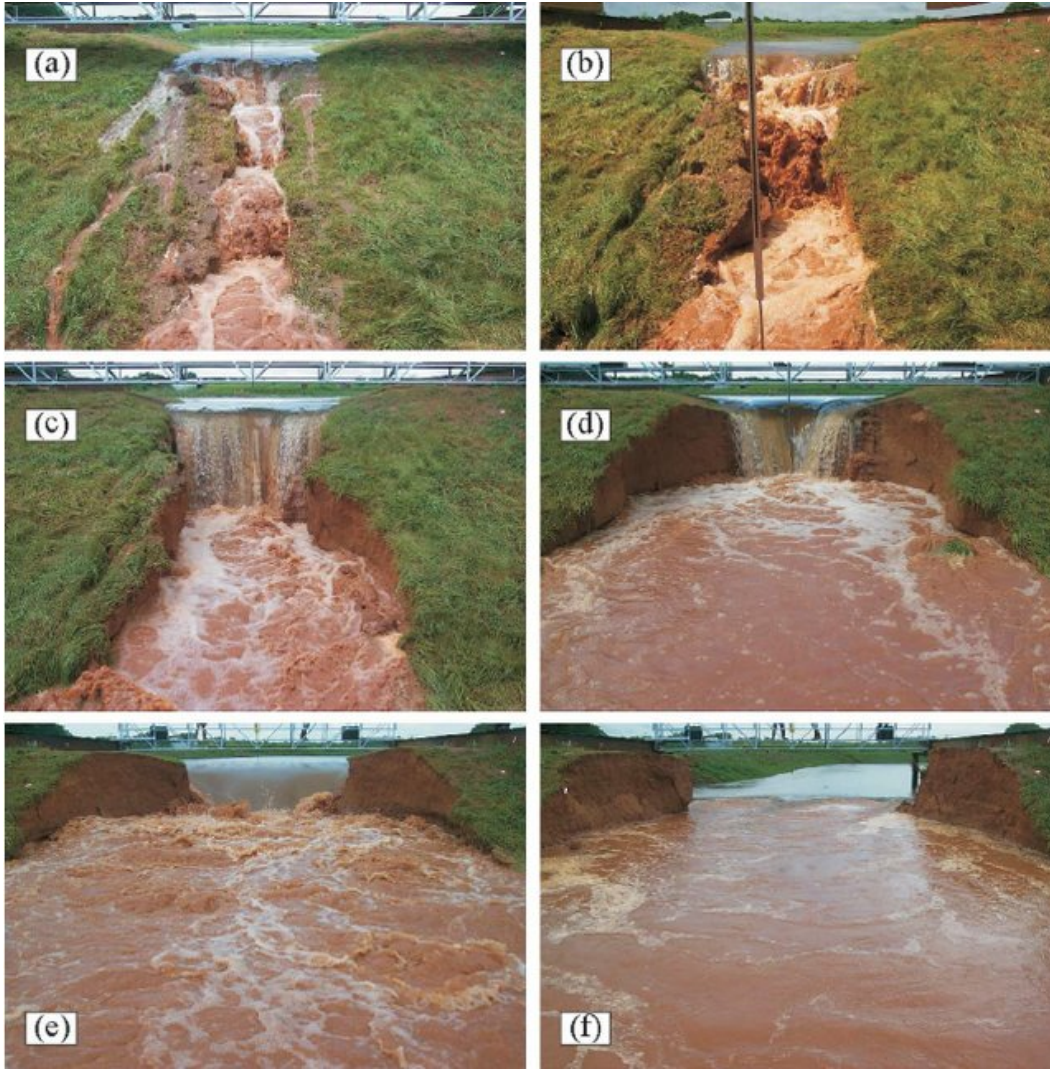
Figure 1-4: An illustration of the dam breaching process by overtopping: (a) rills and cascade of small overfalls at t = 7 min; (b) consolidation of small overfalls at t = 13 min; (c) headcut at downstream crest at t = 16 min; (d) headcut at upstream crest at t = 31 min; (e) flow through breach at t = 40 min; (f) transition to final breach stage at t = 51 min [14].
